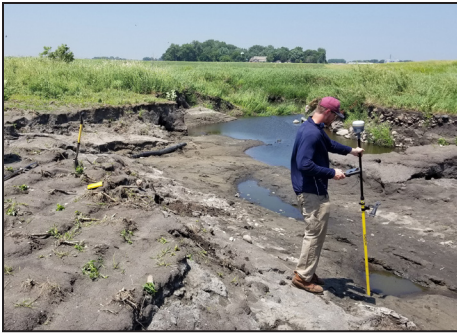
Left: Civil engineering technician Brian Jacobs surveyed a large gully along Butterfield Creek in Watonwan County. A rock chute was later installed at the site to allow water to flow in and out of the creek during high water events. Middle: South Central TSA senior civil engineering technician Greg Schemmel surveyed the site of an embankment failure in Sibley County using a total station, a surveying instrument that measures distances, angles and coordinates. Right: South Central TSA engineer Ryan Jones assessed erosion in a ravine channel downstream from a potential project site in Sibley County.
