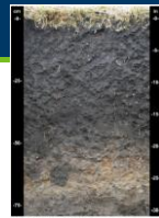
Figure 11. Indicator A12 (Thick Dark Surface). This observation is needed to determine whether a soil meets the requirements of the indicator in the field setting in the laboratory.
