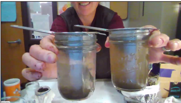
University of Minnesota Extension Educator Anne Sawyer performed a slump test during the session “Learning from Critters: Soil Biology and Interpreting Indicators: Part I,” on Oct. 27 during BWSR Academy. Slump tests compare how the same type of soil under different management conditions behaves when saturated. Photo Credits: BWSR
