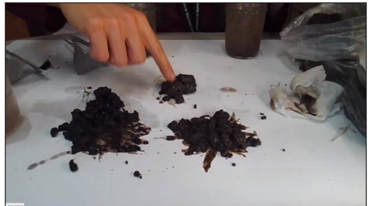
University of Minnesota Extension Educator Anne Sawyer performed a slump test during the session “Learning from Critters: Soil Biology and Interpreting Indicators: Part I,” on Oct. 27 during BWSR Academy. Slump tests compare how the same type of soil under different management conditions behaves when saturated. Photo Credits: BWSR
