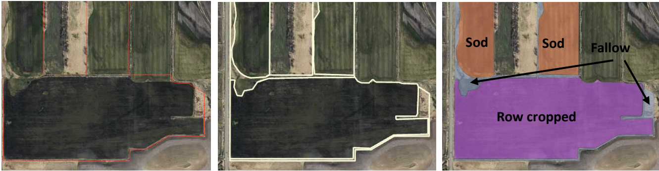
Figure 14. Example of a site stratified by pre-construction land use, resulting in three monitoring units (row cropped, sod, and fallow). Additional monitoring units would be created if multiple plant communities are expected in one or more of the three.
